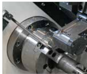
Chuck Air Blow (Upper Chuck)
