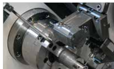
Chuck Air Blow (Upper Chuck)
