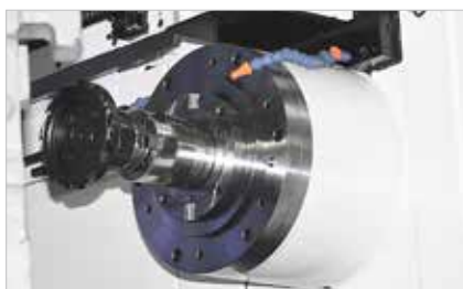
Spindle Nozzle & Cutting Air Blow
